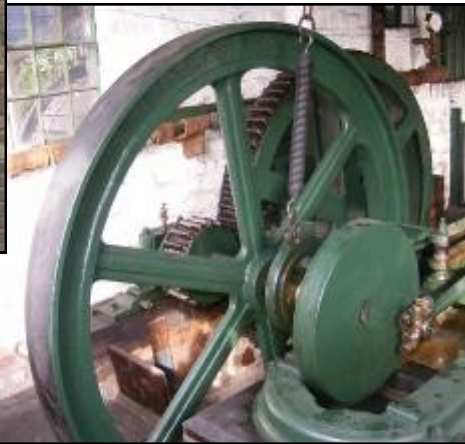
At the back of the Engine House is the large drum which held the wire rope that ran over the wheel at the top of the head frame
