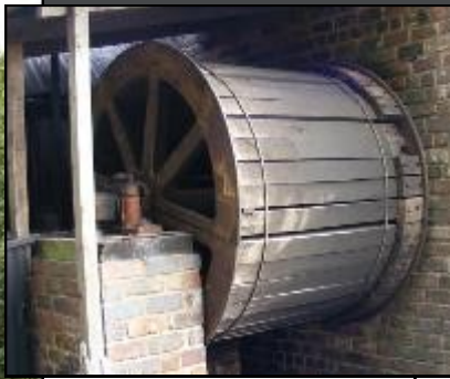
At the back of the Engine House is the large drum which held the wire rope that ran over the wheel at the top of the head frame
